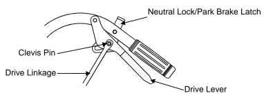
FIG. 9 LEVER AND ROD ADJUSTMENT
